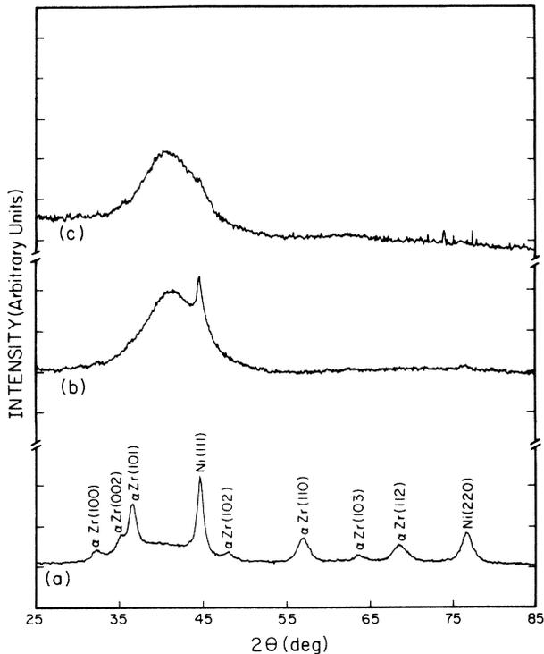
FIG. 3. X-ray diffraction profiles (Cu  $K\alpha$  radiation) for the bulk sample of Fig. 1(c), a multilayered composite of Ni and Zr of average stoichiometry  $\text{Ni}_{66}\text{Zr}_{34}$ . (a) The as-co-deformed sample. (b) The sample after being heated at 10 K/min to a temperature of 675 K and quenched to room temperature in the differential scanning calorimeter. (c) The sample after being annealed at a temperature of 600 K for 4 h and quenched to room temperature.
