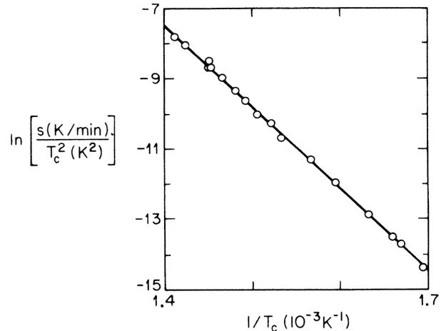
FIG. 4. The natural logarithm of the heating rate,  $s$ , divided by the square of the crystallization temperature,  $T_c$ , vs the inverse crystallization temperature. The solid line is a least-squares fit to the data points.
